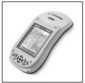
The next step up is mapping accuracy equipment. The unit pictured here is a Trimble unit very similar to what NeRWA uses in our mapping projects. The accuracy of this equipment is improved when the data is corrected, which we do, and usually around 80% to
