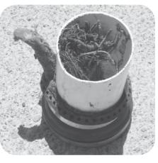
were a couple of rubber boot connectors for sewer
