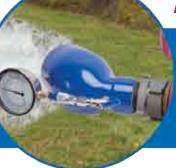
2<sup>1</sup>/<sub>2</sub>" Flow Testing Diffusers include a gauge so you can easily measure flow during hydrant flushing. A built-in baffle and rotating head let you control discharge pressure and direction.
